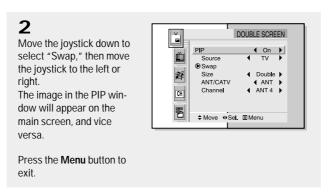
Note: When the selection of ANT-B or Component mode is made, the PIP Swap function doesn't work.
